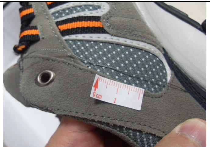
44_minor defect-untrimmed thread end
