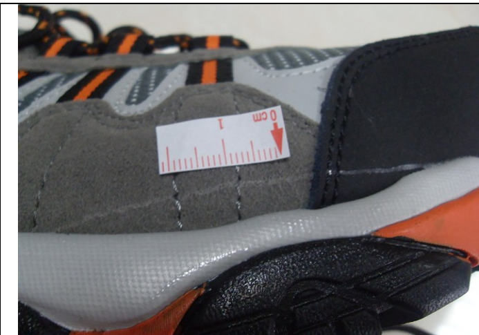
45_minor defect-glue marking on product
