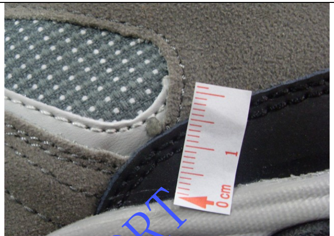
46_minor defect-glue marking on product
