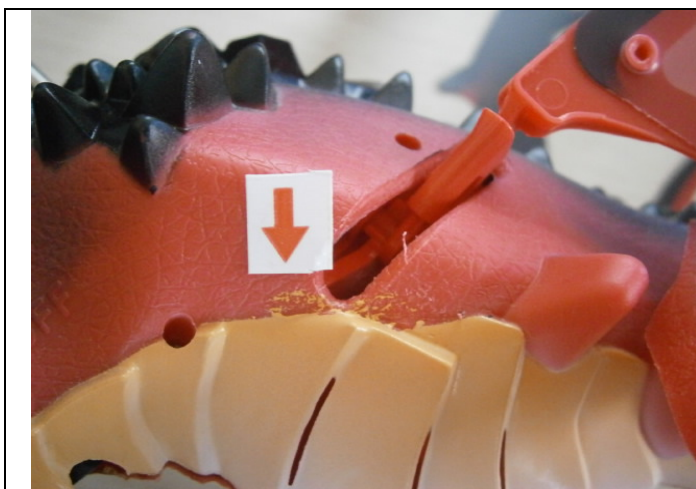
125_minor defect-color stain (2)
