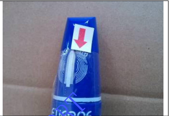
68_defect-missing printing on the product-ma
