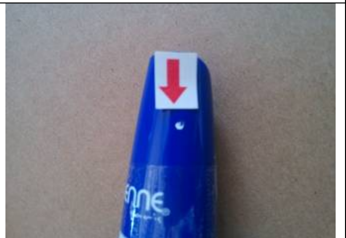
84_defect-extra printing at the head-ma
