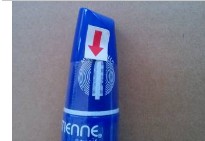
67_defect-missing printing on the product-ma
