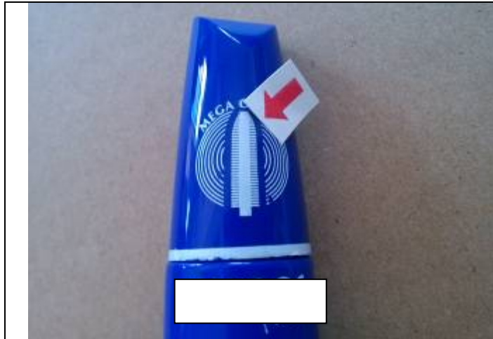
73_defect-missing printing on the product-ma
