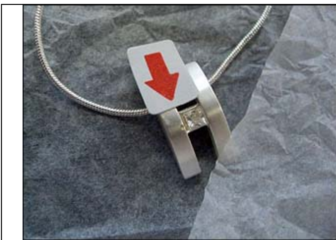
25. Minor defect-Glue mark on surface of product
