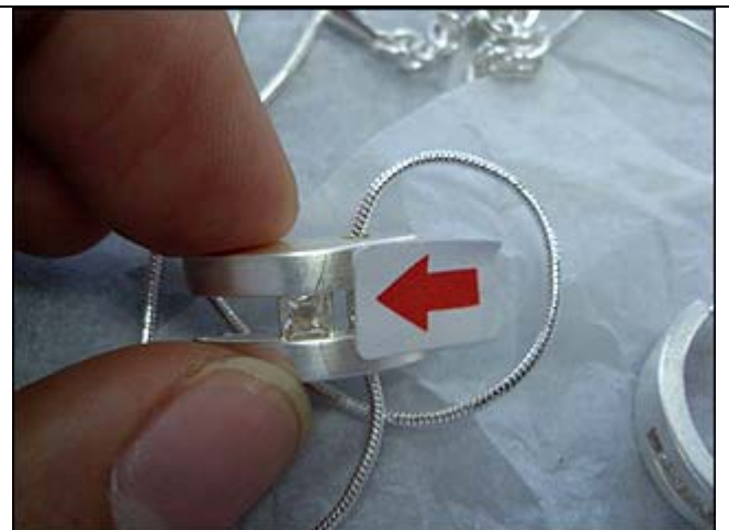
24. Minor defect-Glue mark on surface of product
