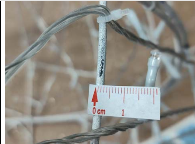
1. Minor defect- Painting peel off of item: 6.736.026
