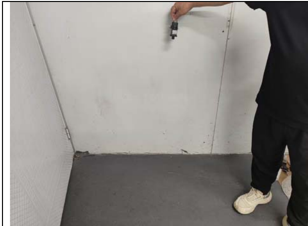
447 Unit drop check for adaptor
